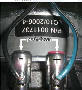
The positive (blue and black) and negative (solid black) cables are still attached to the woofer terminals. Remove the cables from their terminals simply by pushing down on the terminal and pulling out the cable.
